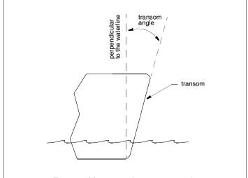
Figure 2. Measuring the transom angle
