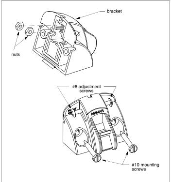
Figure 3. Installing the adjustment and the mounting screws
