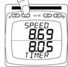
Press to resynchronise to nearest full minute (8:00)
